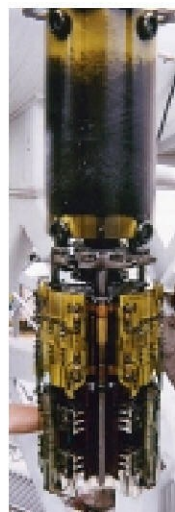
Diverter switch with carbon deposits
