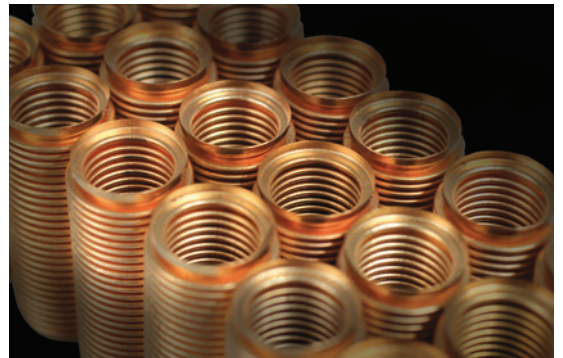
In the MESSKO® BeTech bellow type technology, the measuring system of the oil and winding thermometers consists of four basic components. In this maintenance-free technology, the first bellows ensures actuation of the micro-switches, the second bellows ensures optimum compensation of the ambient temperature.
